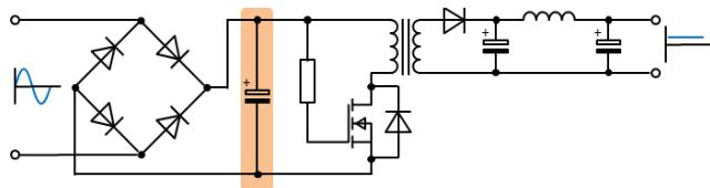
*Fig. 1: Input smoothing capacitor in a Flyback SMPS*
