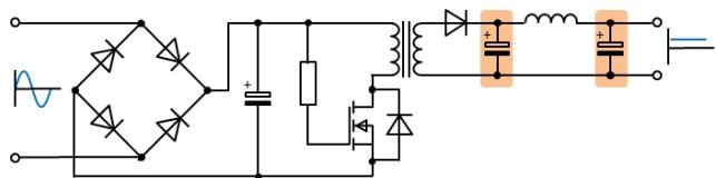
*Fig. 2: Output smoothing capacitors in a Flyback SMPS*
