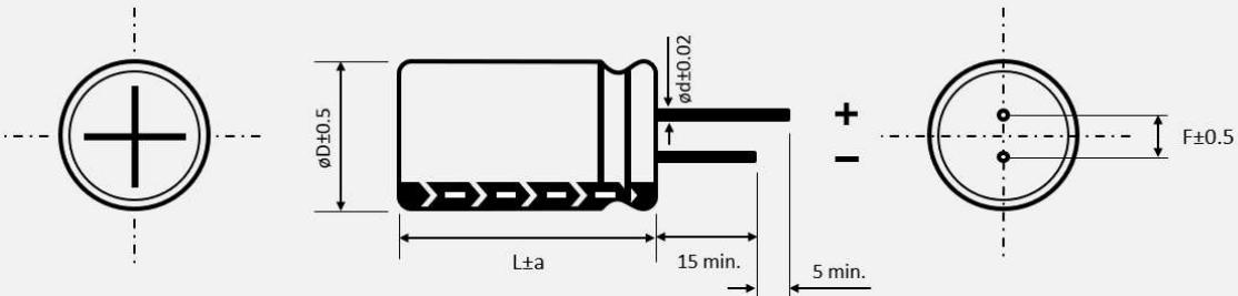
Radial type • CA version - cutted leads - standard lead spacing
